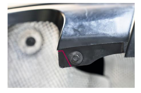
The rear bumper requires trimming for the L/H outlet. The red line on the 1st image indicates the position.
