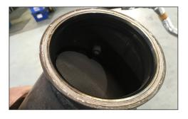
Gasket: Remove the gasket from the original downpipe and re-install on the Scorpion downpipe
